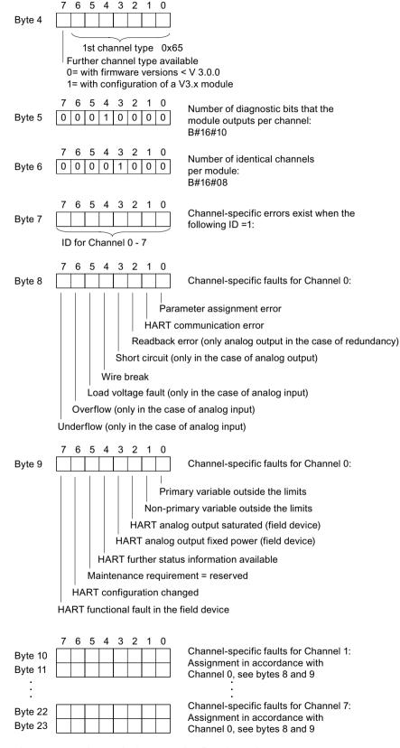
Figure 7-4 Diagnostic data record 1, first channel type
