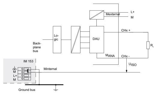
Figure 2-6 Connection of loads to a current output of a HART-AO
