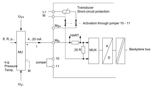
Figure 2-3 Connection of a 4-wire transducer (4...20mA) to a module configured for a 2-wire transducer (4...20mA)
