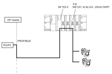
Figure 1-1 Forwarding parameter assignment data with an IM153-2 and HART analog modules
