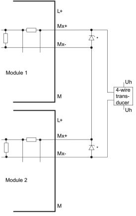
\* Zener diode 5.1 V (e.g., BZX85C5V1), only required if a module is removed and the system should continue running.
