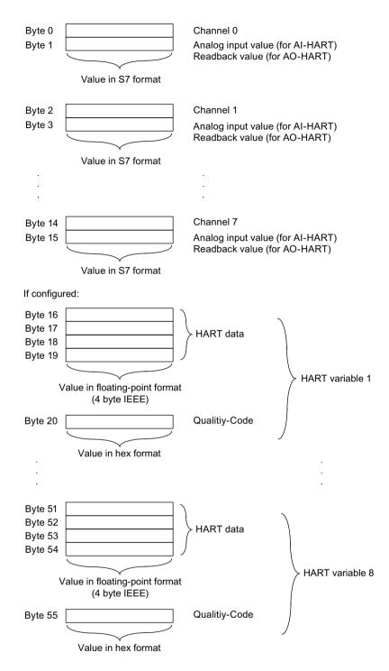
Figure 7-9 Input user data area of the HART analog modules
