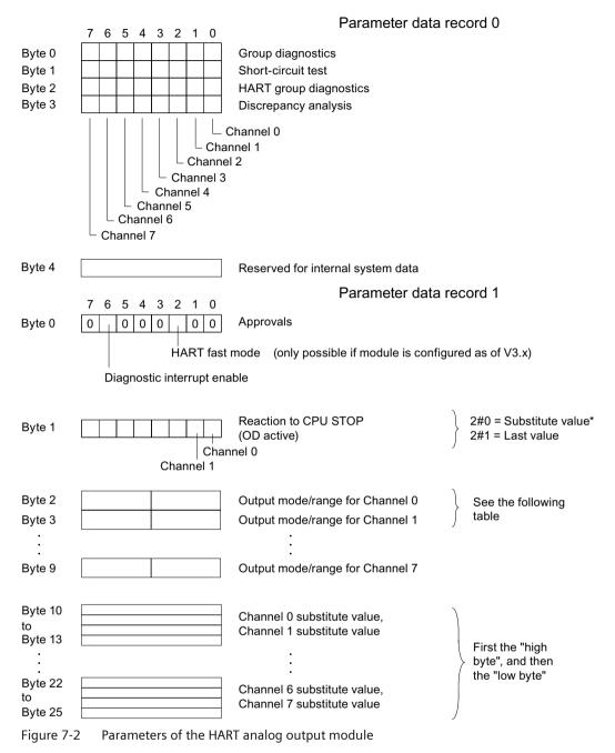
\* With a substitute value of -6912 (E500 Hex) the outputs are deenergized.
