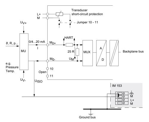
Figure 2-4 Connection of 4-wire transducers to a HART-AI
