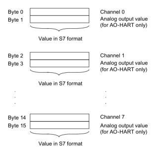
Figure 7-10 Output user data area of the HART analog modules
