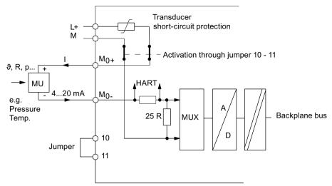
Figure 2-2 Connection of 2-wire transducers to a HART-AI
