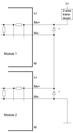
\* Zener diode 5.1 V (for example BZX85C5V1), only required if a module is removed and the system is to continue running.
