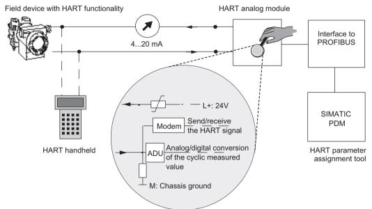
Figure 2-11 System environment for the use of HART
